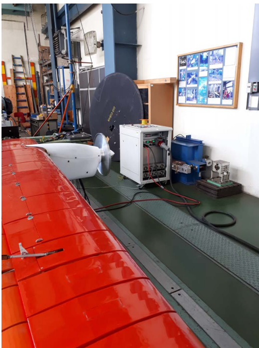
Fig. 3: Complete model OMA, configuration with propeller substitute disc.
