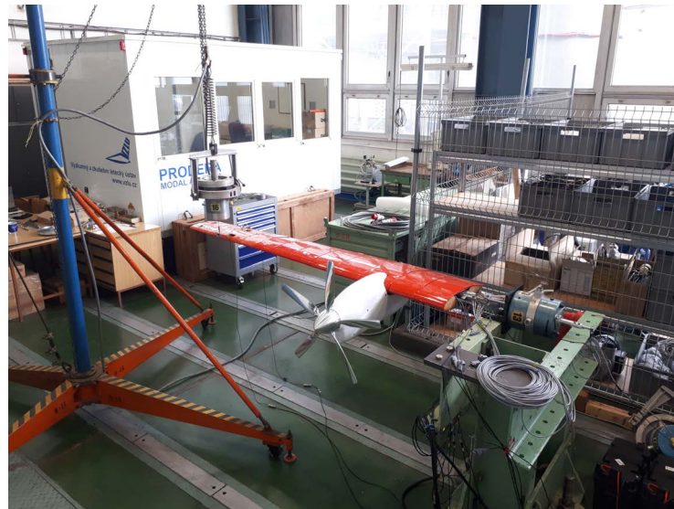
Fig. 2: Complete model modal test arrangement.
