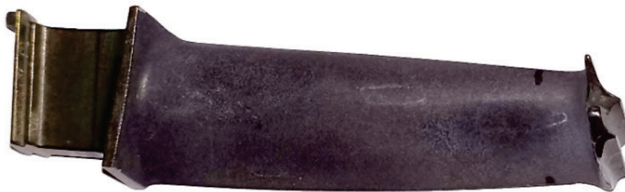
Fig. 1: The turbine blade after the service life
