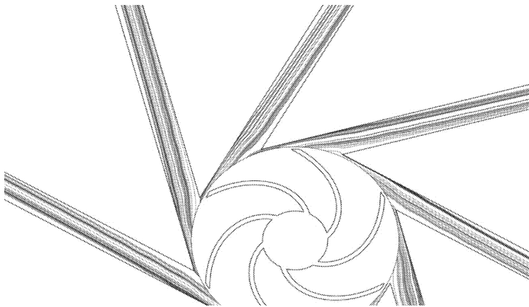
Fig.13: Streamlines in a cross-section of the middle of the stator chamber (stator channels with straight channels inclined by 15^\circ )
