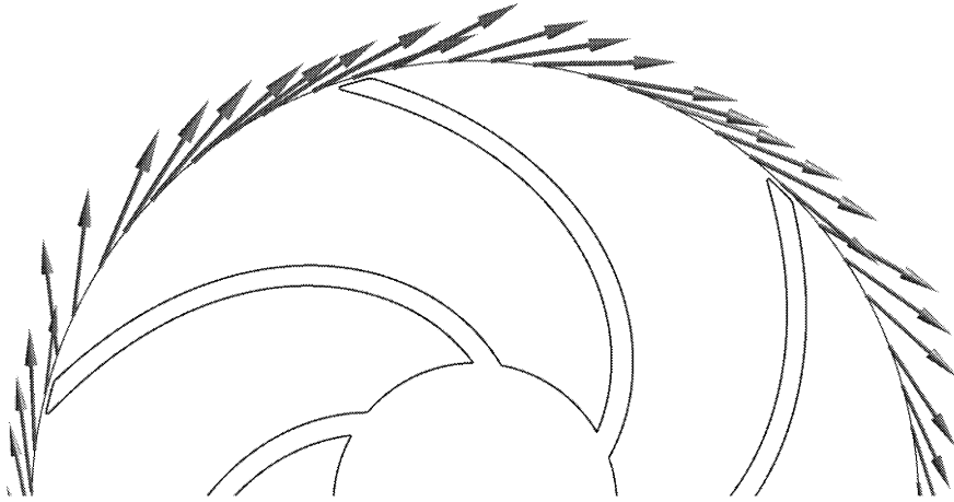
Fig.9: Absolute velocity vectors in a cross-section through the middle of outlet width and cylindrical surface
