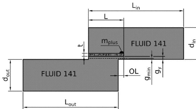
Fig.1: Parametric model with changeable parameters and corresponding finite element types
