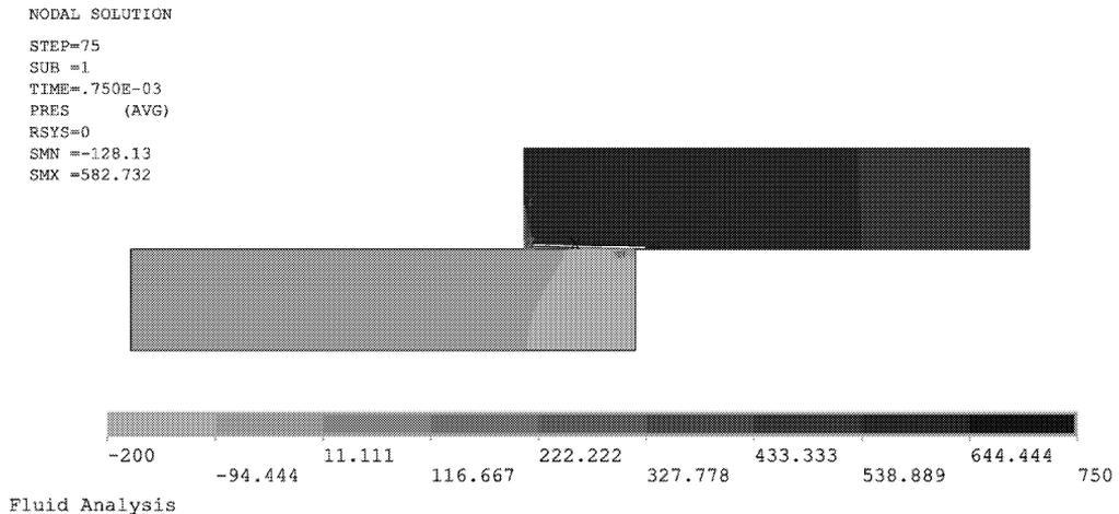
Fig.5: Acoustic pressure at  $t = 0.75 \times 10^{-3}$  s in Pascals
