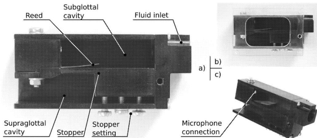
Fig.9: Experimental model
