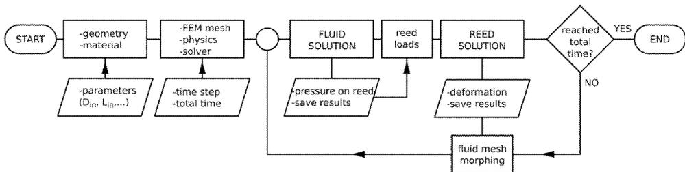
Fig.3: Algorithm flowchart
