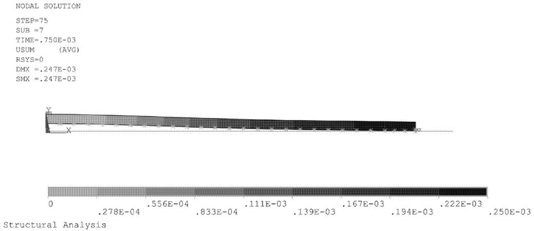
Fig.4: Reed deformation at  $t = 0.75 \times 10^{-3}$  s in millimeters (reed-stopper contact occurred)
