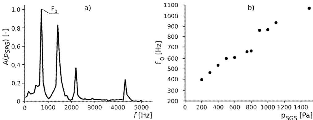
Fig.6: a) Frequency spectrum  $p_{SPG}$  for inlet pressure  $p_{SGS} = 500$  Pa
