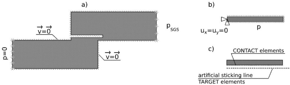
Fig.2: Boundary conditions prescribed to the reed and the air cavity boundaries
