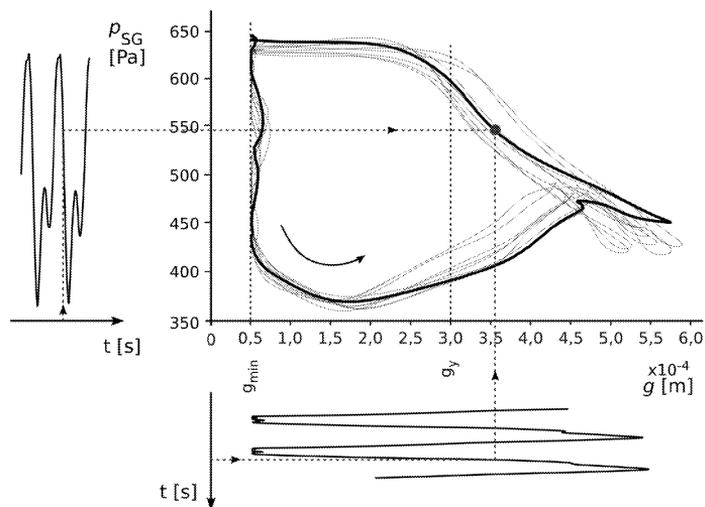
Fig.7: Method of  $g$ - $p_{SG}$  diagram construction
