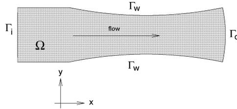
Fig.2: Solution domain – nozzle
