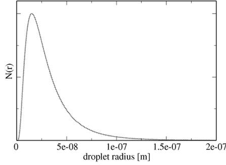
Fig.1: Example of log-normal droplet size distribution
