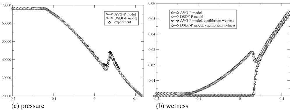
Fig.3: Pressure and wetness along nozzle axis, experimental data from [2]
