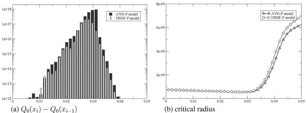
Fig.4: Increments of number of droplets  $Q_0(x_i) - Q_0(x_{i-1})$  and critical radius  $r_c$  within the nucleation zone in grid points  $x_i$
