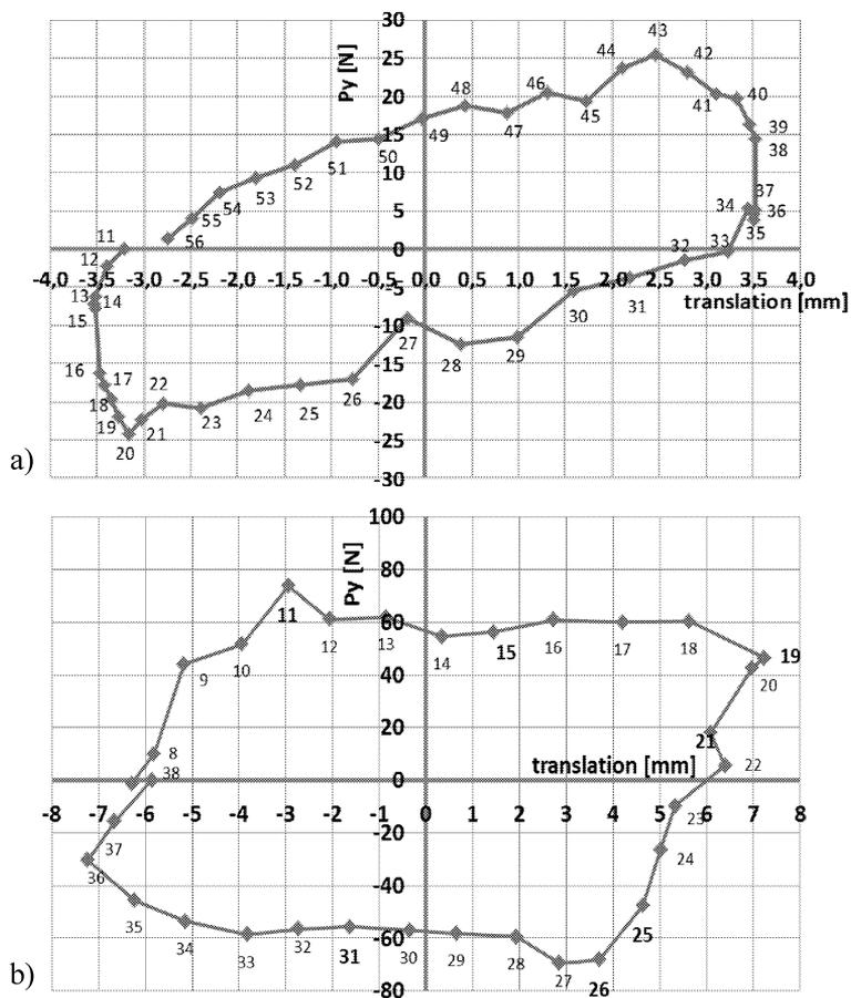
Fig.4: Total lifting force as a function of profile translation : a)  $M = 0.21$ ; b)  $M = 0.45$
