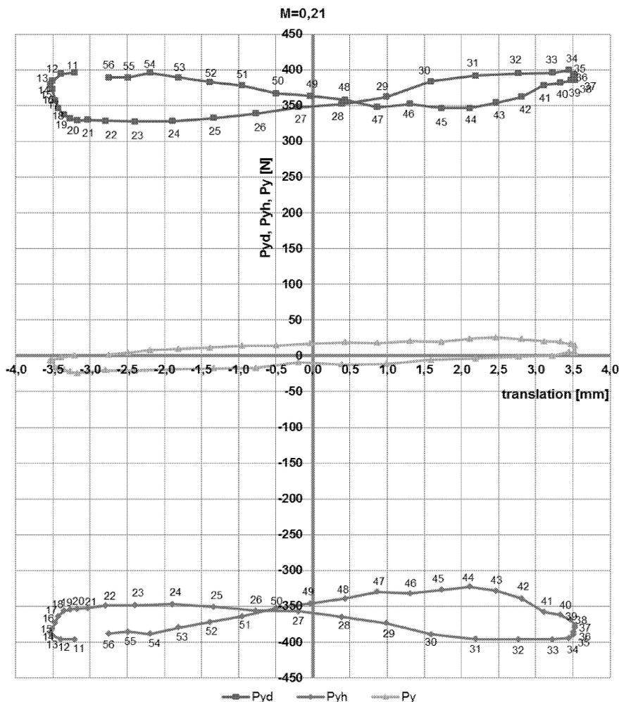
Fig.5: The lift as the function of the translation ( $M = 0.21$ ,  $P_{y,d}$  - lower,  $P_{y,h}$  - upper surface of the profile)
