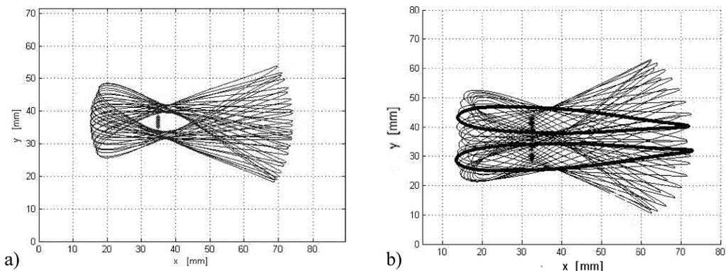
Fig.2: Profile positions during one period of flutter: a)  $M = 0.21$ ; b)  $M = 0.45$
