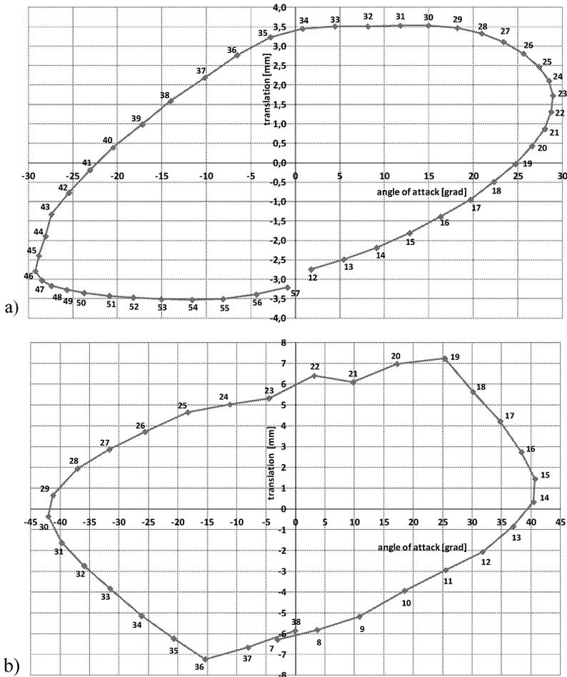
Fig.3: Translation as the function of the angle of attack during one period of flutter: a)  $M = 0.21$ ; b)  $M = 0.45$
