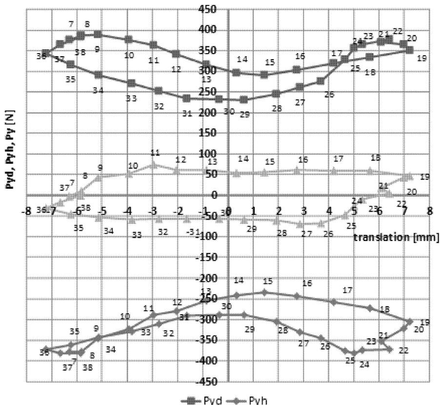
Fig.6: The lift as the function of the translation ( $M = 0.45$ ,  $P_{yd}$  – lower,  $P_{yh}$  – upper surface of the profile)
