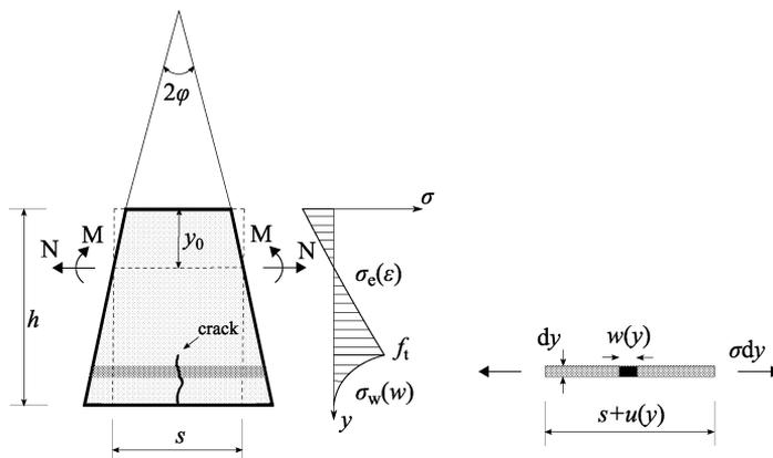
Fig.1: Loading and deformation of the cracked hinge element with a stress distribution (left) and incremental layer inside the hinge considered as the single non-linear spring (right)
