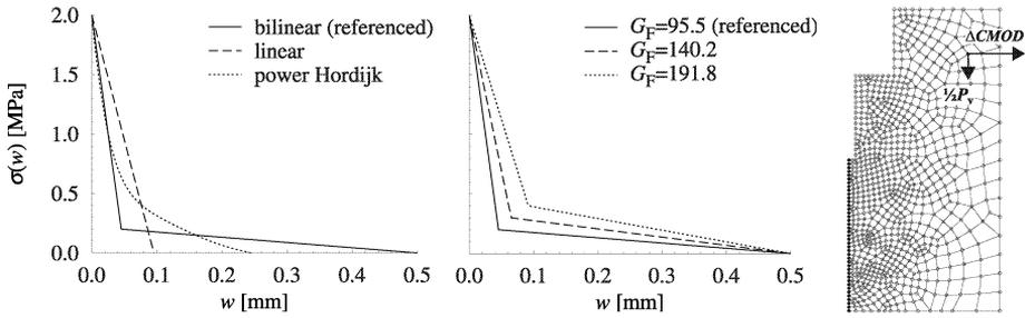
Fig.3: The defined tensile softening functions: with constant (left) and increasing (middle) values of the fracture energy; FE mesh of the WST specimen (right)
