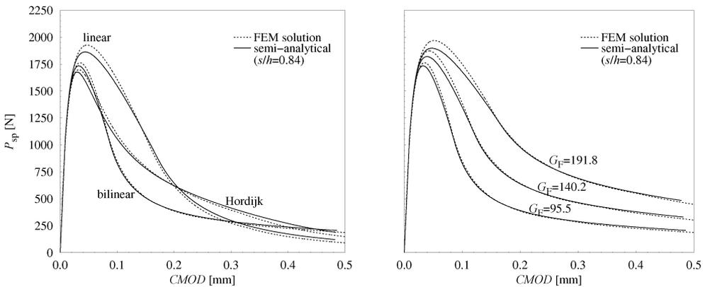
Fig.5: Simulated  $P$ - $CMOD$  diagrams of the models using the defined tensile softening functions with the constant (left) and increasing (right) fracture energy
