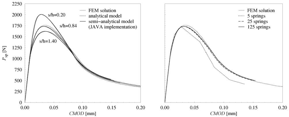
Fig.4: Simulated  $P$ - $CMOD$  diagrams of the models using the defined tensile softening functions with the constant (left) and increasing (right) fracture energy
