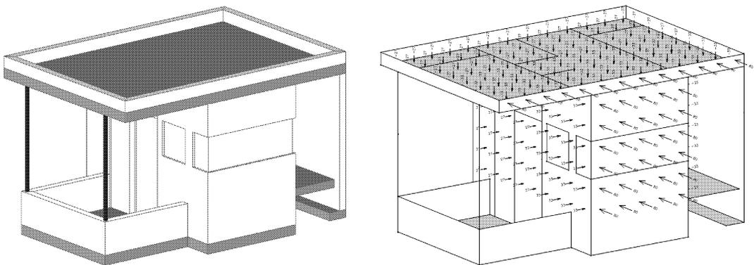
Fig.1: Calculation model of the whole structure (North-West view) and dynamic forces in selected points of above-ground parts
