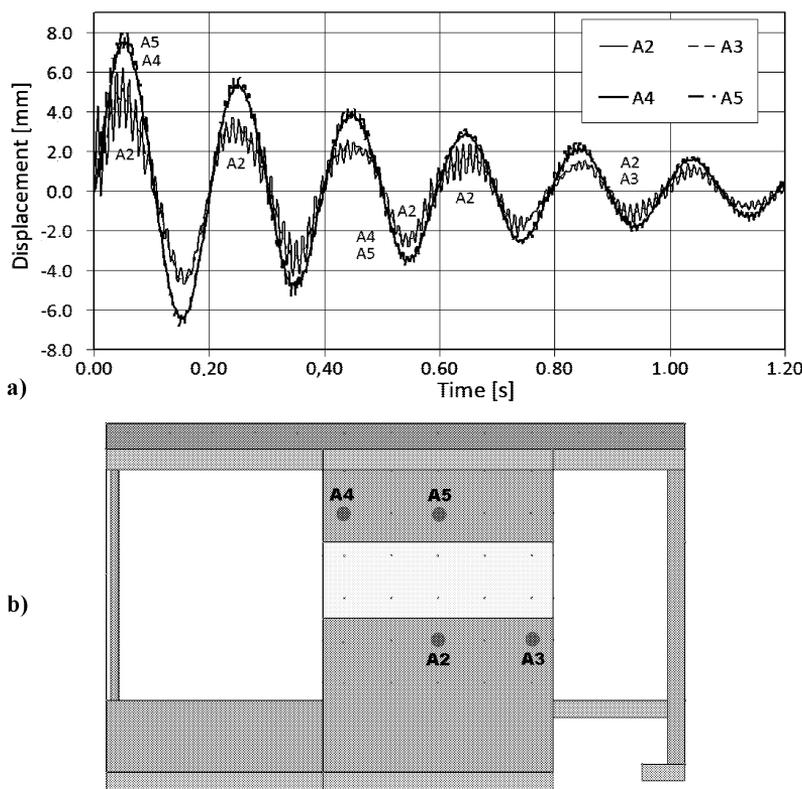
Fig.2: Time history of vibration (a) in selected points (b) of front wall
