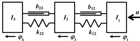
Fig.3: Serial structure of electronic cam
