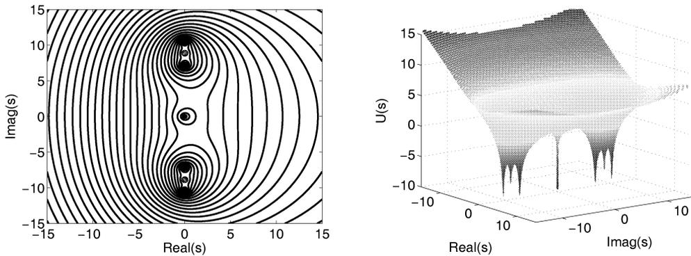
Fig.11: Spectral analysis of 9<sup>th</sup> order polynomial shaper
