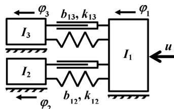
Fig.5: Parallel structure of electronic cam
