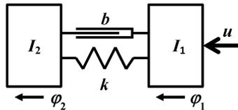
Fig.2: Two-mass model of the electronic cam
