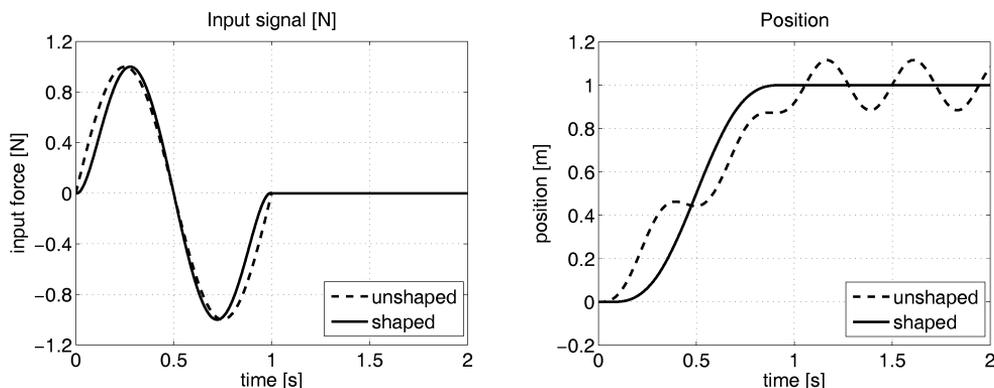
Fig.1: Comparison of shaped and unshaped control input
