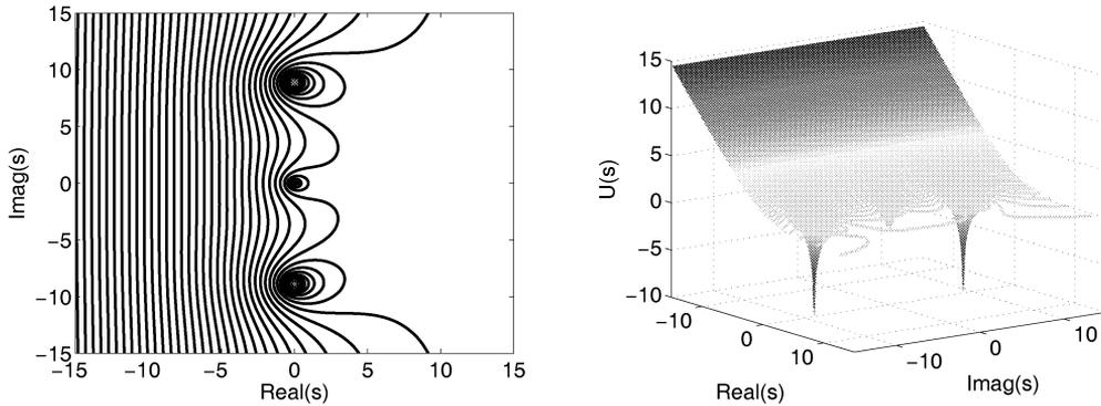
Fig.10: Spectral analysis of 7<sup>th</sup> order polynomial shaper
