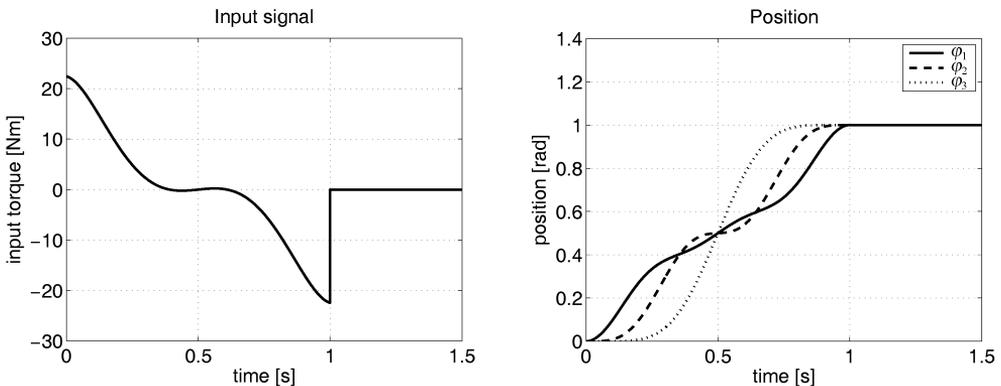
Fig.6: Parallel electronic cam – shaped input and system response
