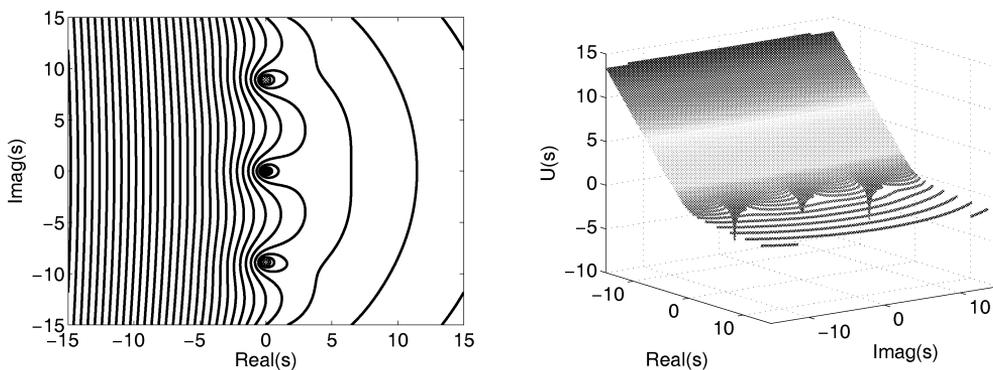
Fig.9: Spectral analysis of 5<sup>th</sup> order polynomial shaper
