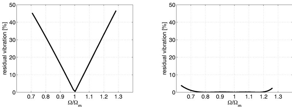
Fig.12: Sensitivity to modelling errors a) 5<sup>th</sup> order shaper b) 9<sup>th</sup> order shaper
