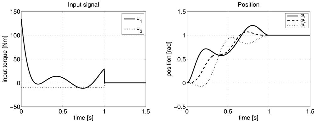
Fig.8: Two-inputs electronic cam – shaped input and system response
