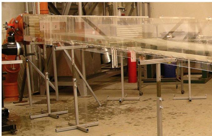
Fig.1: Overall view of the water open channel with one rib
